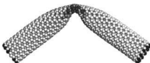
FIGURE 1.9 MD simulation of a large-amplitude transverse deformation of a carbon nanotube, apparently beyond the elastic limit. In fact, the tube snaps back once the computer-generated force is removed, and there is no plastic deformation or permanent damage. (From Yakobson, B. I., Appl. Phys. Lett. 72 , 918–920 (1998), with permission.)
